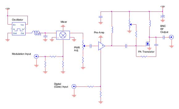
Figure 2: Driver Block Diagram
