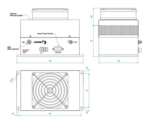
Figure 1: Driver Installation (Driver shown with Fan Option)
