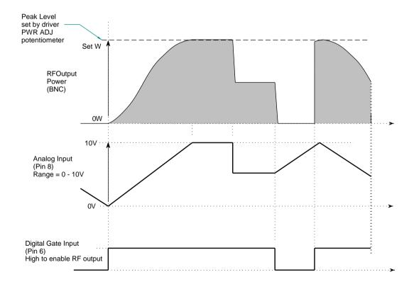
Figure 3: Typical Analog Modulation Waveforms
