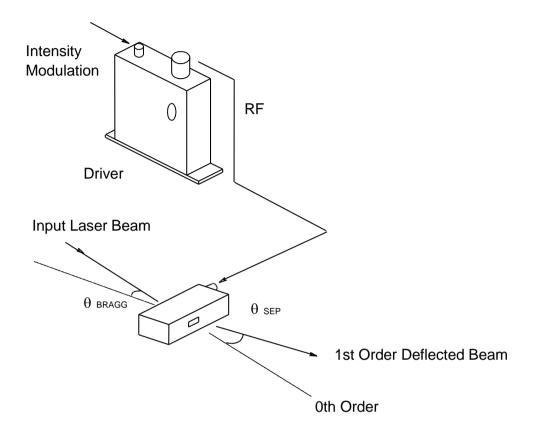
The input Bragg angle, relative to a normal to the optical surface and in the plane of deflection is:
